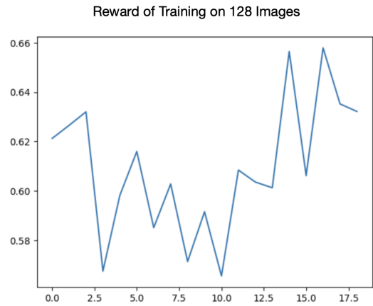
Figure 8: The plot of the average reward of fine-tuning the vision language model on 128 images using the image-text retrieval reward function. After 16 iterations, the model improved the average reward from 0.621 to 0.658.
